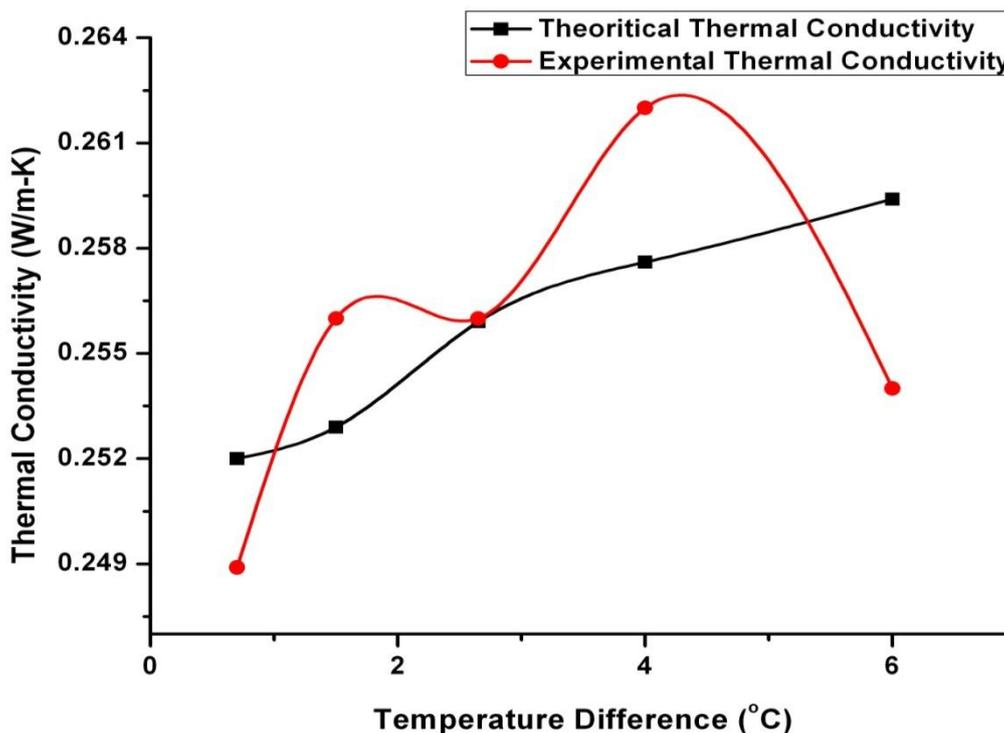
Fig.6 Thermal Conductivity of Ethylene Glycol
