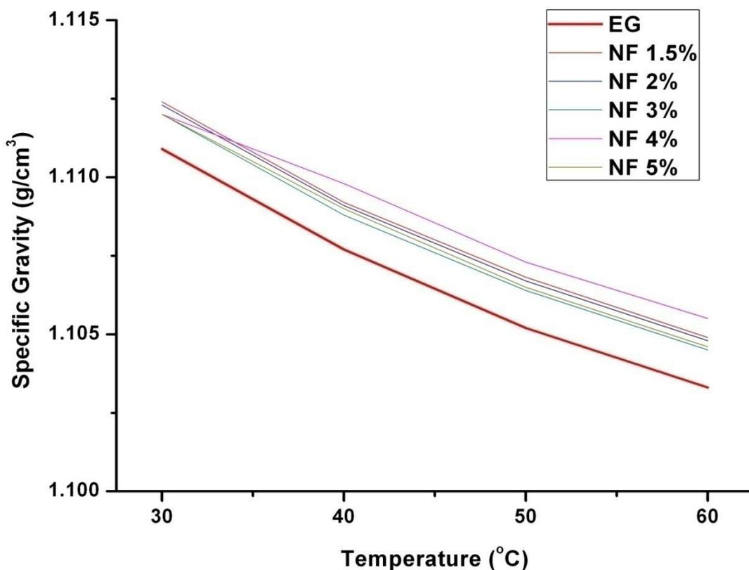
Fig.9 Temperature vs. Specific Gravity of  $\text{In}_2\text{O}_3$  nfs
