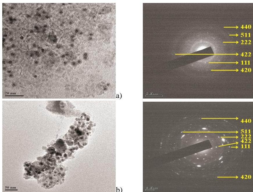
**Fig.4 TEM and SAED pattern of (a) 1:2 (Sample 1) and (b) 1:5 (Sample 2) of  $In_2O_3$  nfs**
