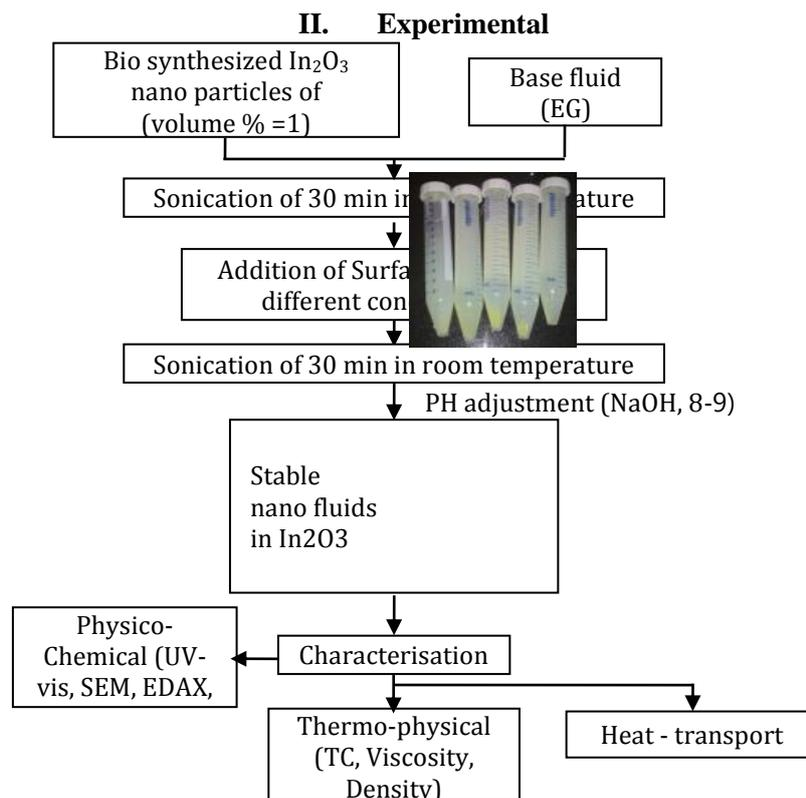
**Fig.1 Flow chart of preparation of  $In_2O_3$  nanoparticles**
