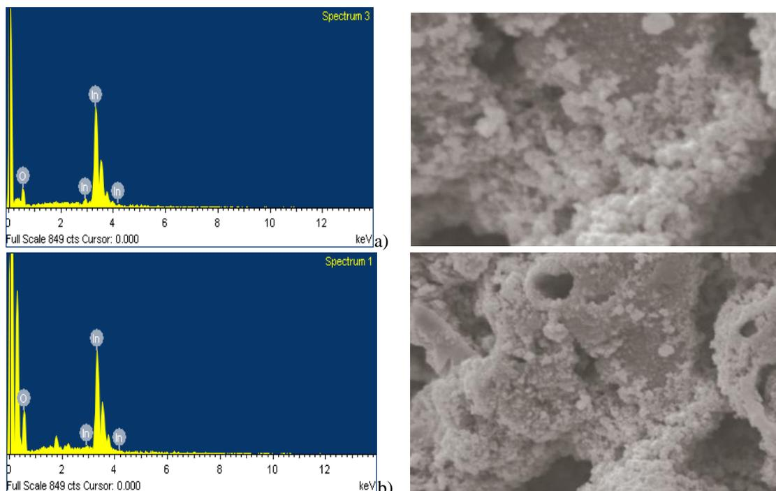
**Fig.3 EDAX and SEM of (a) 1:2 (Sample 1) and (b) 1:5 (Sample 2) of  $In_2O_3$  nfs**
