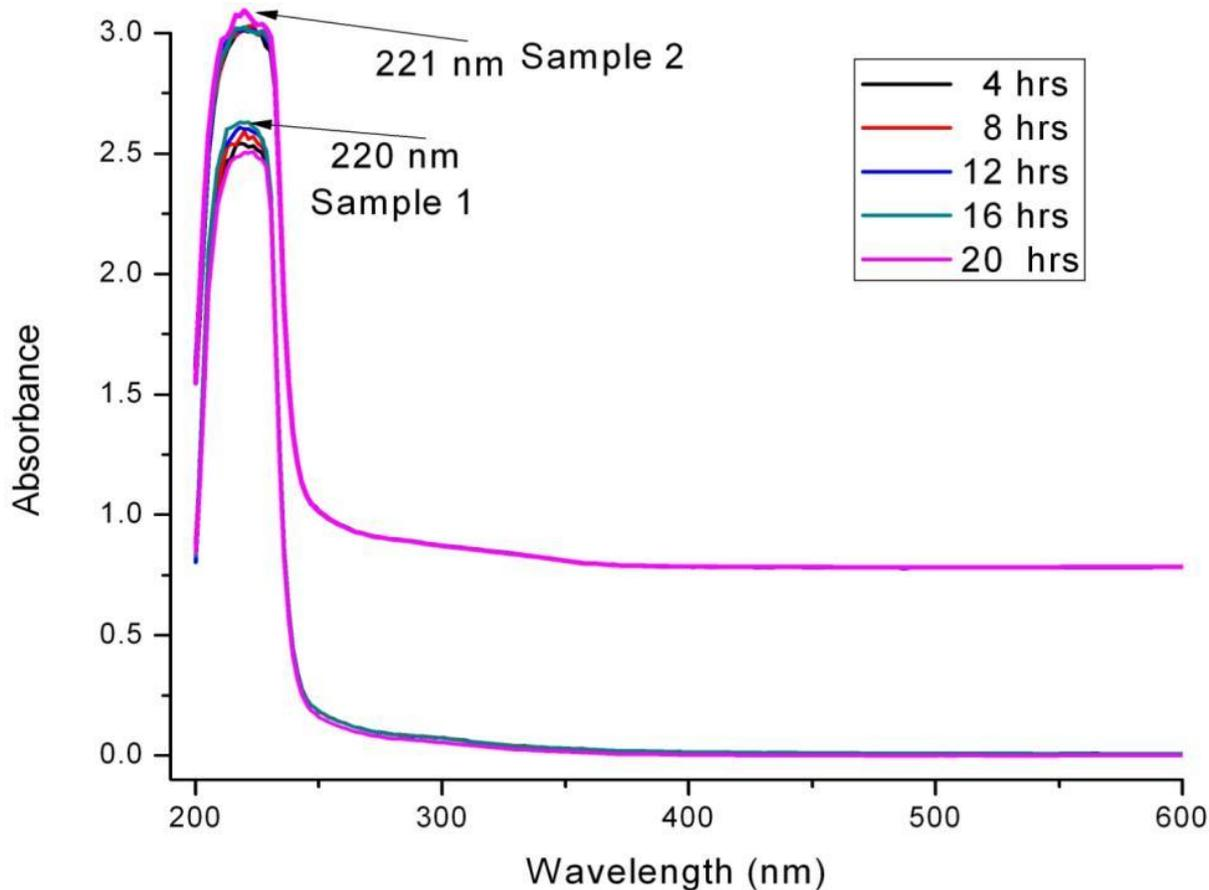
**Fig.2 UV-Vis absorption Spectrum of 1:2 (Sample1) and 1:5 (Sample 2) of  $In_2O_3$  nano fluids**
