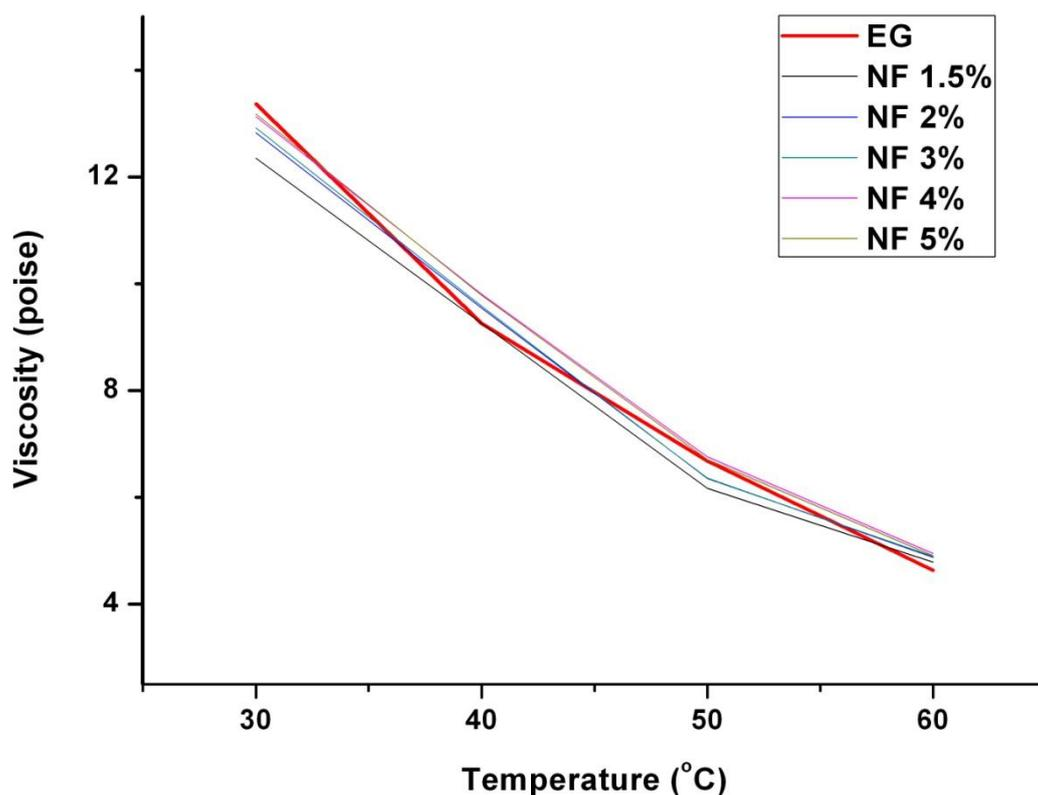
Fig.10 Temperature vs. Viscosity of  $In_2O_3$  nano fluids
