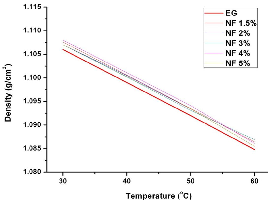
Fig.8 Temperature vs. Density of  $\text{In}_2\text{O}_3$  nfs
